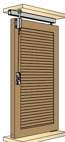
Two possible mounting positions: Mounting on sill or mounting on lintel
